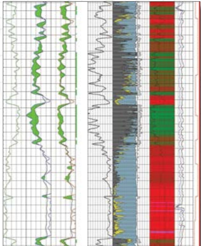
*For additional flexibility in reservoir evaluation, Allied-Horizontal can combine the Reservoir Analysis Sonde (RAS) with other production logging and evaluation tools. Run with the Spectral Gamma Ray Tool, RAS data improves Clay Volume calculations and correlations with Total Organic Content (TOC), making this tool combination ideal for shale gas plays.*
