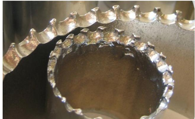
The chemical (Bromine Trifluoride) is then forced through an oil/steel wool mixture, placed at the top of the severing head. The BF<sub>3</sub> chemical reacts with the oil and ignites the steel wool.
